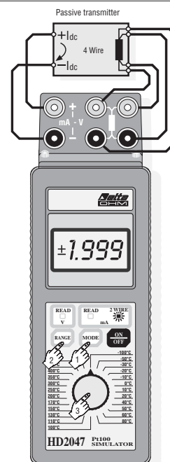
Fig. 3 Testing a Pt100 input passive transmitter
