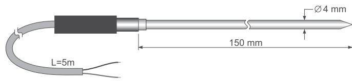
**TP 32MT.12:** T type thermocouple temperature probe, Ø 4mm,L=300mm, 5m cable, isolated. Temperature range -40...+100°C.
