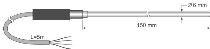
**TP 32MT.11P:** T type thermocouple temperature probe, Ø 4mm,L=150mm, pointed, 5m cable, isolated. Temperature range -40...+100°C.
