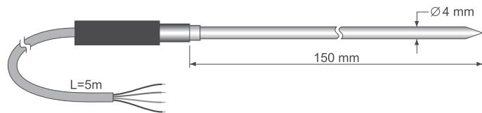
**TP 32MT.2I:** 4-wire 1/3 DIN Pt100 temperature probe, Ø 6mm,L=150mm, 5m cable, isolated sensor. Temperature range -40...+100°C.
