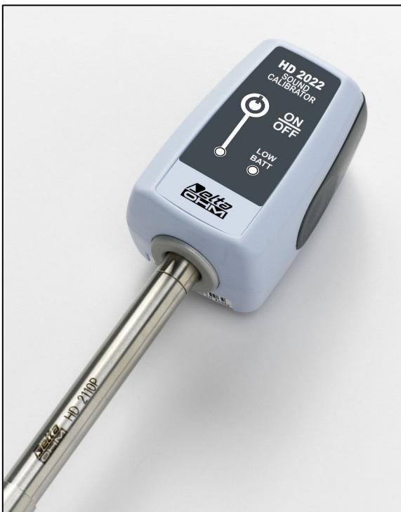
The HD2022 sound level calibrator is a portable, battery operated sound source, suitable for sound level meters (portable and laboratory) and acoustic stations.
